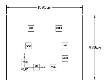
Die Size: 1095 μm X 930 μm (Not Drawn To Scale)
